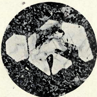
3.—Quartz. Ordinary Light. Showing corrosion.
